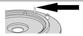
If you have lifted up the hotplate then carefully replace it taking care not to damage or displace the ignition electrodes or flame safety probes (arrowed) and replace the rear fixing screws.
